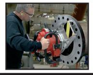
The SDB series and EP 424 are great tools for refinishing raised face flanges. Wachs tooling is designed with the necessary geometry to create a raised face record groove finish on most materials. Wachs flange facing tool kits include everything required to machine the full range of flanges within each machine's capacity. Replacement tooling inserts are ideal for this application and feature three cutting surfaces to maximize tool life.
