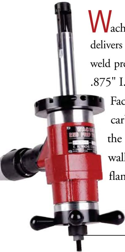
**W**achs SDB 103/3 is a hand held beveling machine that delivers maximum power and performance for fast, accurate weld preps. The machine operates on pipe and tube from .875" I.D. through 4.5" O.D. (22.2mm to 114.3mm).
