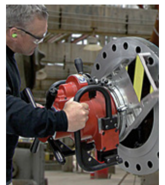
Ideal for facing flanges when properly equipped
