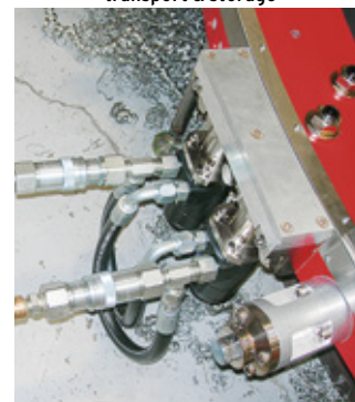
LDSF standard dual hydraulic drive motors & dual pinion housings
