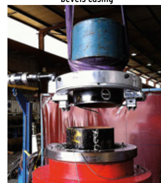
ECC can be inverted for cuts low to the wellhead
