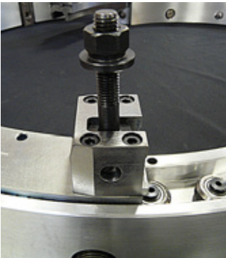
Aluminum stationary frame with steel rotating ring
