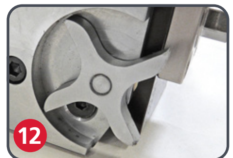
12 No-time starwheel tool advance is designed to work with the anti-crash trip
