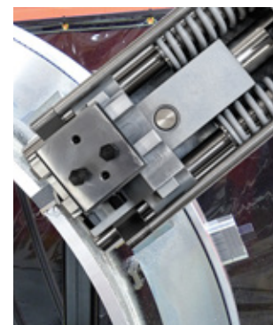
OD tracking slides follow out-of-round pipe & vessels.
