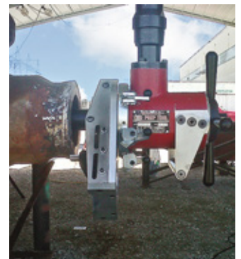
SDB end prepping pressure vessel
