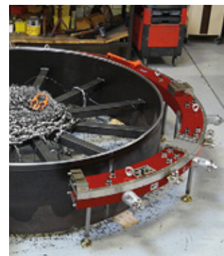
Four standard LDSF sizes cover 60-120in (DN1500-3000)
