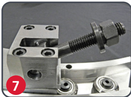
7 Swing bolts allow for fast positioning over inline pipe
