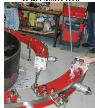
LDSF splits into quadrants for setup, transport & storage
