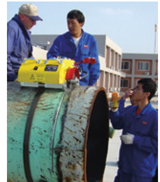
Trav-L-Cutter is designed for pipeline operations.
