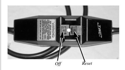
Figure 5-6. Press the reset button on the GFI to power on the electric WAVE handheld.
