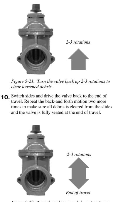
Figure 5-22. Turn the valve up and down two times against the end of travel to fully seat it in the closed position.
