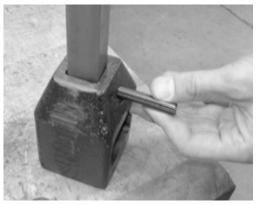
Figure 5-1. Install the socket onto the end of the valve key and insert the pin through the socket and key.
