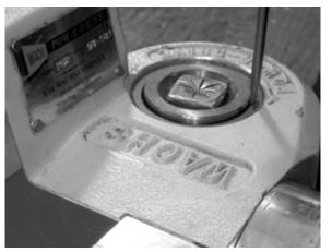
*Figure 7-1. Pry out the old oil seal with a flat-blade screwdriver.*
