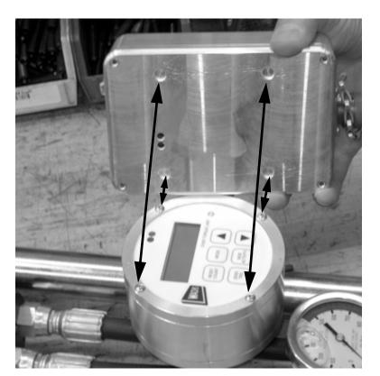
Figure 5-36. Aligning the VITALS<sup>TM</sup> data logger with the WAVE<sup>TM</sup> handheld control unit. The four holes in the back of the data logger fit onto the screws on the face plate of the control unit.
