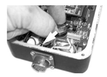
Figure 3-22. Remove the old battery from the socket.
