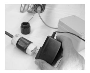
Figure 3-13. Plugging in the charger will start charging the battery.
