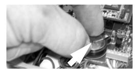
Figure 3-18. Slide the new battery into the socket, with the plus side (+) up.
