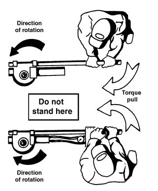
Figure 5-5. The operator should always stand so that the handle of the WAVE<sup>TM</sup> machine pulls away from his body.
