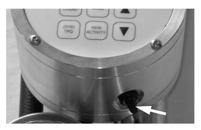
Figure 7-7. Control unit power switch (hydraulic and pneumatic systems only). Press the button and release it to toggle the control unit on and off.
