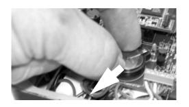
Figure 3-17. Remove the old battery from the socket.
