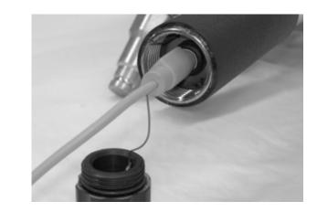
*Figure 3-12. Charger plugged into the battery charg*ing connector. Note that the connector must be aligned correctly to line up the pins with the sockets.
