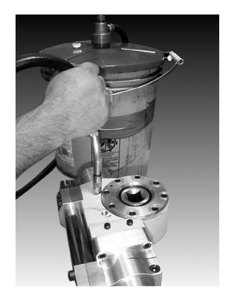
Figure 6-2. Adding oil to the gearbox.
