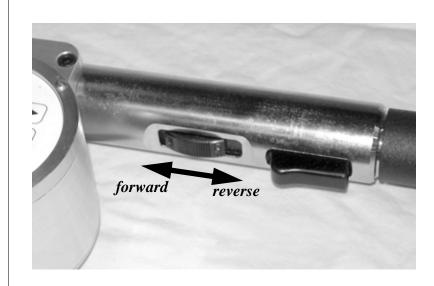
Figure 5-10. Set the direction of rotation using the direction control switch. The forward position sets the rotation in the right-hand direction. The reverse position sets the rotation in the left-hand direction.
