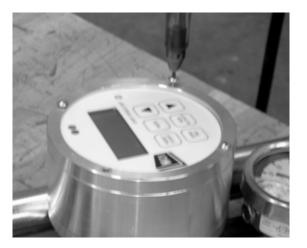
Figure 7-8. Remove the screws on the control unit face plate to open the control unit.
