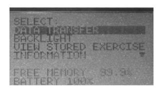
Figure 3-8. Data logger system menu. Use the up and down arrow buttons to highlight the options. Scroll past the bottom of the menu to display the second screen of commands. Press the NEXT button to select the highlighted option.
