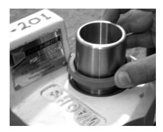
Figure 7-3. Slide the seal down onto the fitting.
