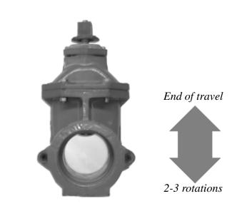
Figure 5-25. Turn the valve up and down two times against the end of travel to fully seat it in the open position.
