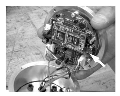
*Figure 7-9. The replaceable battery is mounted in a socket on the control unit circuit board.*
