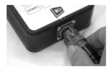
*Figure 3-19. Plug the charger cable into the VITALS<sup>TM</sup> connector.*
