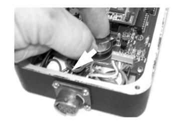
Figure 7-13. Remove the old battery from the socket.
