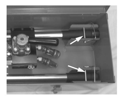
Figure 4-1. Insert the pins to secure the WAVE handheld system and the extension handle into the storage case.
