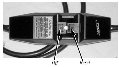
Figure 7-6. Press the Off button on the GFI to power down the electric WAVE handheld.
