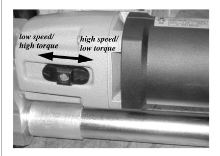
Figure 5-11. The speed switch is on the bottom of the electric motor housing.
