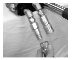
Figure 5-7. Attach the return hydraulic hose first. (The photo shows quick-fit connectors installed. These connectors are optional, or you can install your own.)
