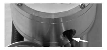
Figure 3-10. Control unit power switch (hydraulic and pneumatic systems only). Press the button and release it to toggle the control unit on and off.
