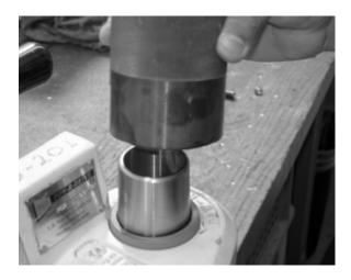
Figure 7-4. Put the appropriate sized sleeve over the press fitting onto the top of the seal.
