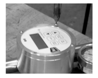
Figure 3-15. Remove the screws on the control unit face plate to open the control unit.
