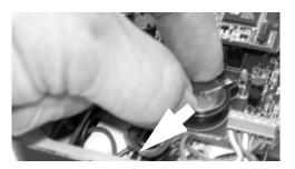
Figure 7-10. Remove the old battery from the socket.
