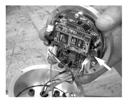
*Figure 3-16. The replaceable battery is mounted in a socket on the control unit circuit board.*
