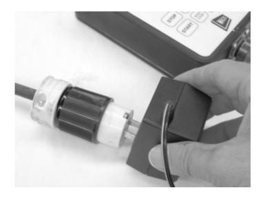
*Figure 3-20. Plugging in the charger will start charging the battery.*
