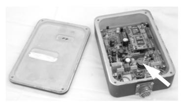
*Figure 7-12. The memory battery is in a socket on the circuit board.*
