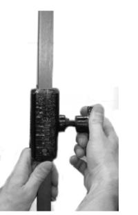
Figure 5-3. Slide the stop collar onto the key and use the set knob to fasten it at an appropriate height.
