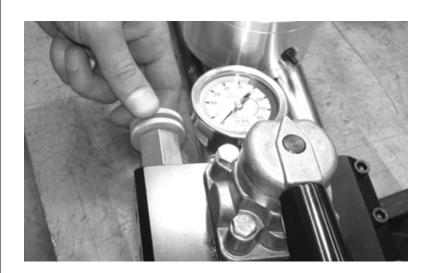
Figure 5-13. Set the torque using the torque controlled knob. Before starting, turn the knob to the lowest torque setting.
