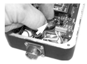
Figure 7-14. Slide the new battery into the socket, with the plus side (+) up.
