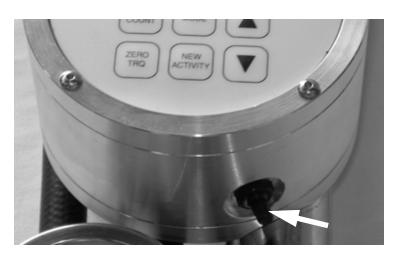
Figure 3-14. Control unit power switch (hydraulic and pneumatic systems only). Press the button and release it to toggle the control unit on and off.
