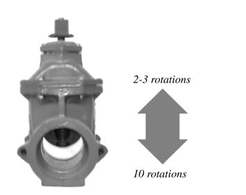
Figure 5-19. Continue driving the valve down. Turn 10 rotations in the closing direction, then 2-3 in the opening direction.
