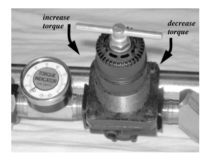
Figure 5-15. Use the air flow valve to adjust the torque.
