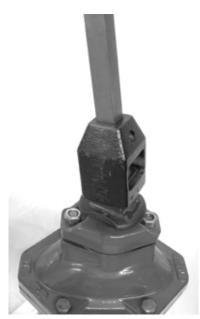
Figure 5-2. Put the socket onto the valve nut.
