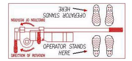
Figure 3-5. Operator position label
