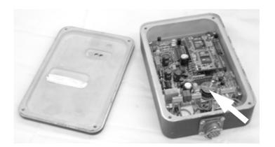
*Figure 3-21. The memory battery is in a socket on the* circuit board.
