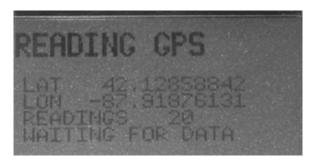
Figure 5-43. READING GPS screen, showing readings for latitude and longitude. (READINGS is the number of GPS data samples integrated by the data logger.)
