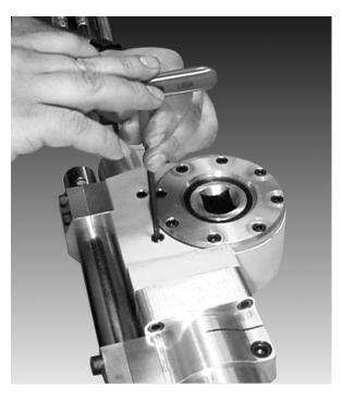
Figure 6-1. Removing the filler and vent plugs.
