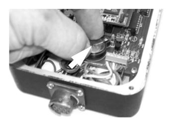
*Figure 3-23. Slide the new battery into the socket, with the plus side* (+) *up.*
