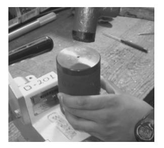
Figure 7-5. Tap the seal into place with a hammer until the sleeve is flush against the housing.
