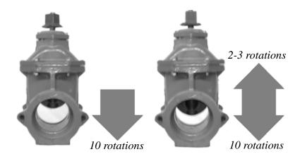
*Figure 3-1. Closing a valve using a "back and forth" process to prevent jamming.*
