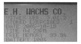
*Figure 5-28. VITALS<sup>TM</sup> data logger power-up screen.*
