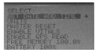
Figure 3-9. Data logger system menu (screen 2). Use the up arrow to scroll back up to the first menu screen.
