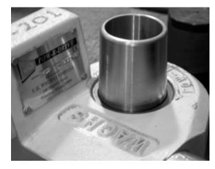
*Figure 7-2. Put the press fitting in place over the bearing.*
