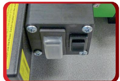
Other Motor Controls include On/Off and Direction
