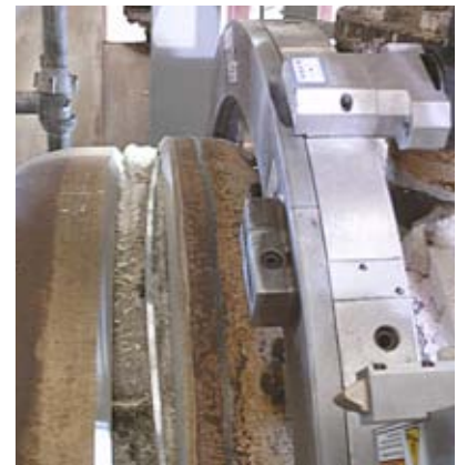
Figure 5 - Out of round tracking slides cut and double bevel
