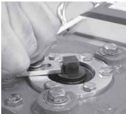
Loosen the lock to turn the spindle feed screw
