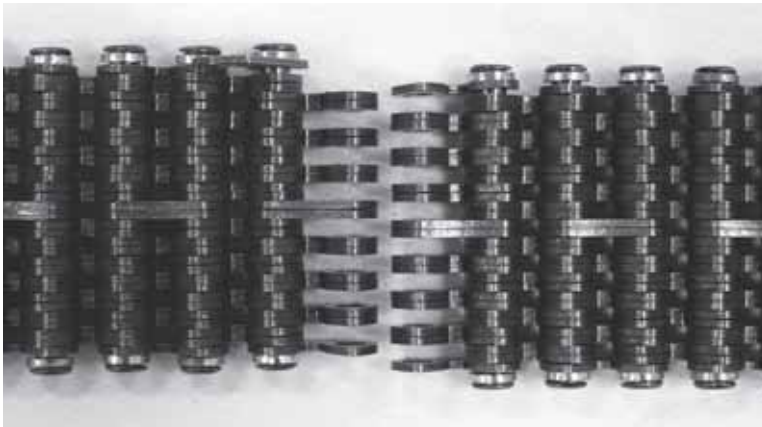
WRONG —Link pins and center links are not aligned
