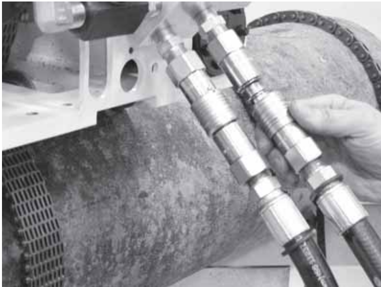
Figure 2-4. Disconnect hydraulic power by removing the hydraulic hoses from the fittings on the machine.
