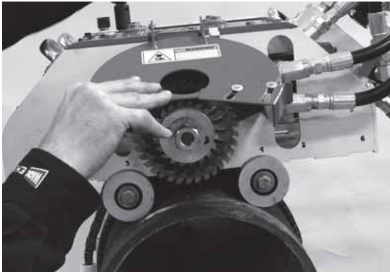
Figure 2-2. The blade guard covers the tooling during operation. Lift the blade guard to install tooling. Always lower the guard over the tooling when operating the machine.
