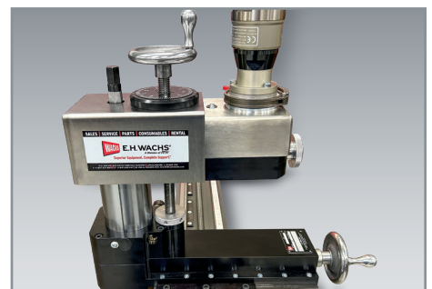
Exchanger Milling Head y-Axis Control (Right) and z-Axis Control (Top)
