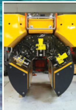
CPT can transit the axis of the pipeline
