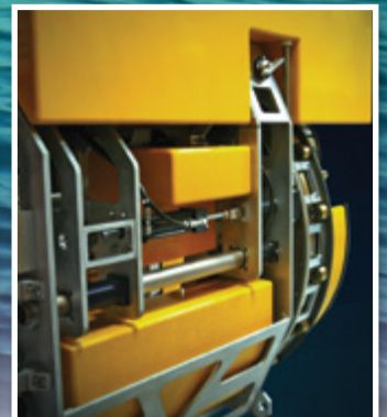
Syntactic foam for neutral buoyancy at depths to 3,000 meters
