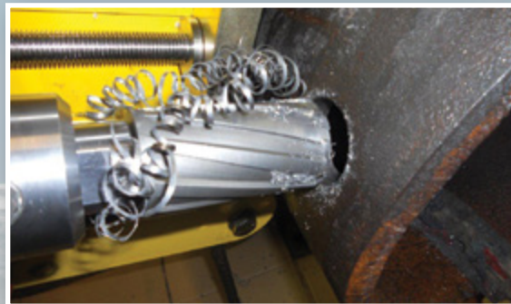
Hydraulically driven variable speed drill is powerful enough to drill a 5in (127mm) diameter hole
