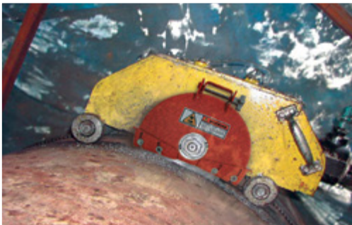
Model HE Trav-L-Cutter operates topside or subsea with its closed loop hydraulic drive system
