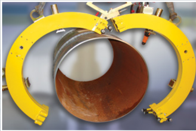
Heavy duty models feature all steel construction for maximum durability and pivot open for ease of positioning
