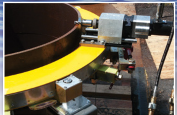
Split frames can be used as cutters or as platforms
