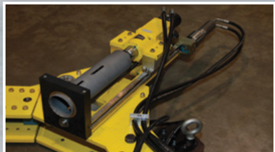
Pin drill spindle motor and feed motor operate separately
