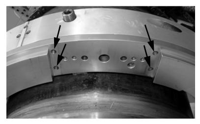
Figure 1-2. There are special holes for the O.D. tracking slides in the LCSF rotating ring at the slide mounting locations.
