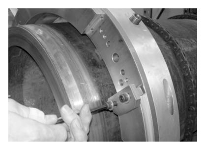
Figure 3-5. Install the mounting clamps on the rotating ring of the LCSF at the slide mounting locations.
