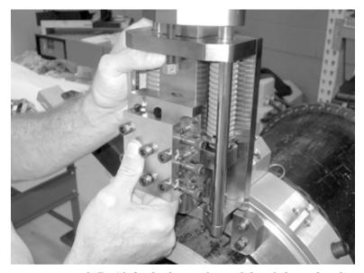
Figure 3-7. Slide the base plate of the slide under the edges of the mounting clamps. Push the slide in all the way until the tracking wheel is against the pipe.
