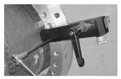
Figure 3-6. Mount the trip on the LCSF with the 3 screws provided.
