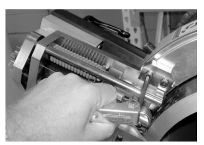
Figure 3-23. Loosen the mounting clamp screws to remove the slides.
