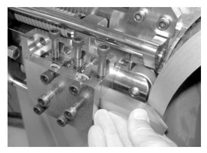
Figure 3-18. Insert the beveling tool into the tool holder as shown.
