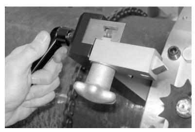
Figure 3-14. Engage the trip by loosening the trip lock lever and pushing the trip bar in toward the LCSF.
