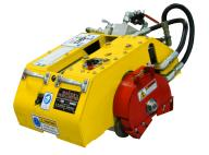
The Wachs Trav-L-Cutter will cut and bevel all common pipe materials, wall thickness and sizes from 6" (DN150) and up. All cutters are manufactured from premium tool steels with exclusive designs to give you consistent quality cutting. Our OEM blades are manufactured and tested to the highest standards in the industry. The cutters listed below are the commonly used tooling for most applications. If you have an application outside of the one's listed please contact us for technical support.
