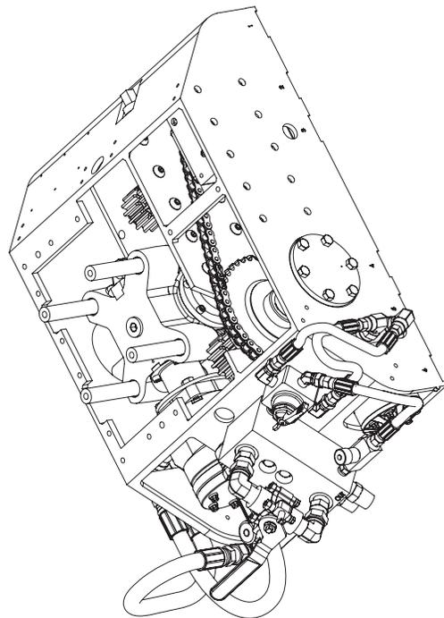
Hydraulic Motor and Frame Assembly
