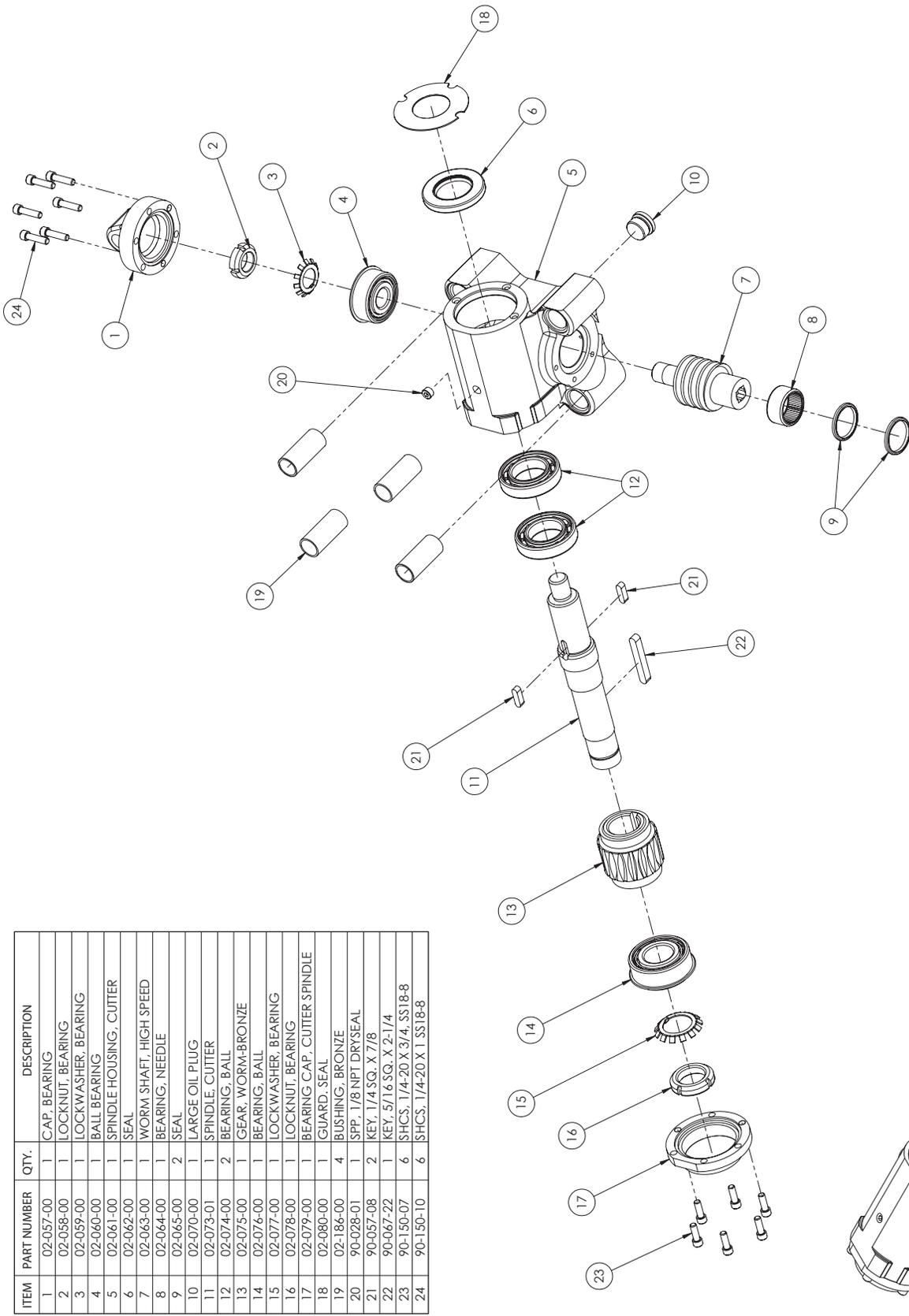
Cutter Spindle Gear Assembly
