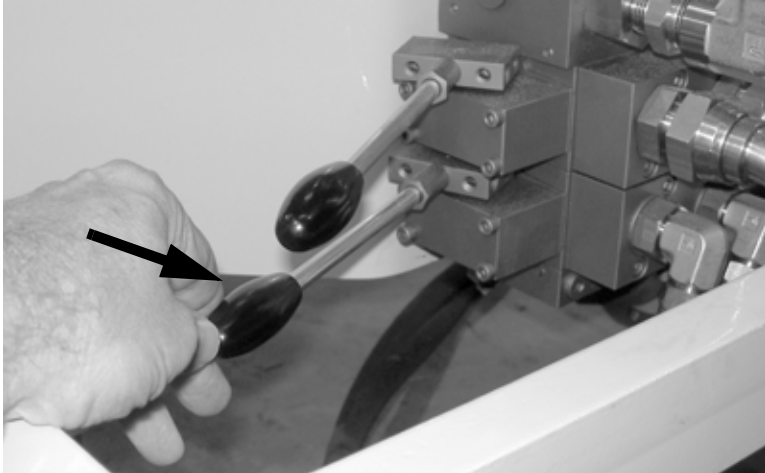
Figure 5-25. Start the feed motion by pushing the bottom lever to the right. The cutting drive lever must be engaged when you do this.
