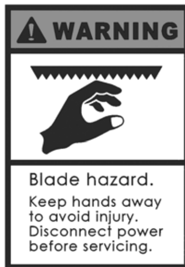
Figure 2-2. Observe the warning label for blade hazard.
