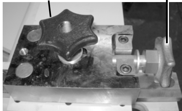
Figure 5-9. The photos show the clamp blocks on the Goliath saw bow. The right block (bottom photo) has a blade tensioning knob.
