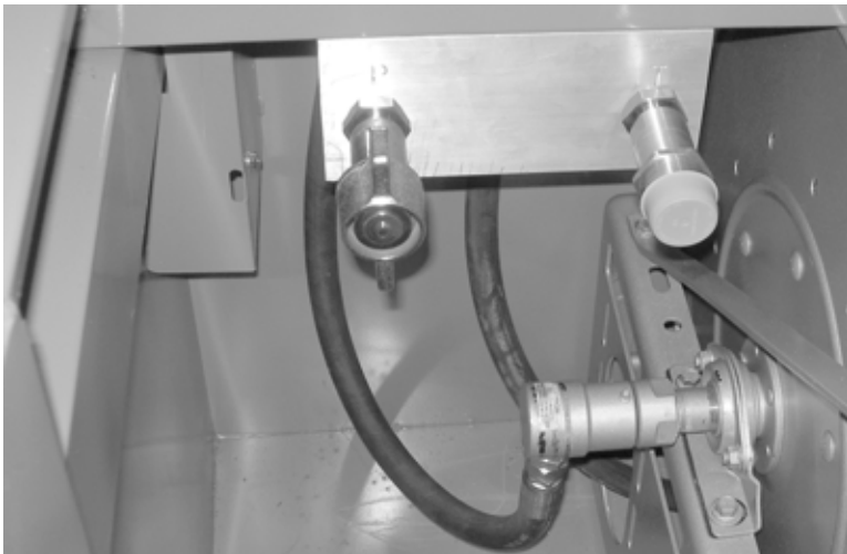
Figure 5-14. Connect the HPU to the hose reel connectors.
