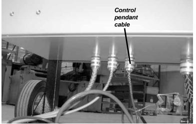
Figure 1-10. Connect the control pendant cable on the bottom of the cabinet.
