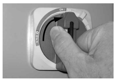
*Figure 1-11. Turn the power switch to the ON position.*
