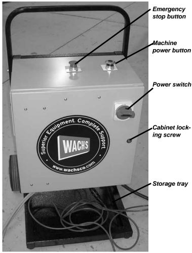
*Figure 1-1. The photo shows the front of the control cabinet.*
