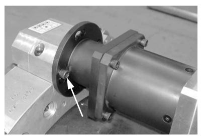
Figure 1-7. Insert the mounting screws and turn the drive to engage them in the slots. Tighten the screws (one each side).
