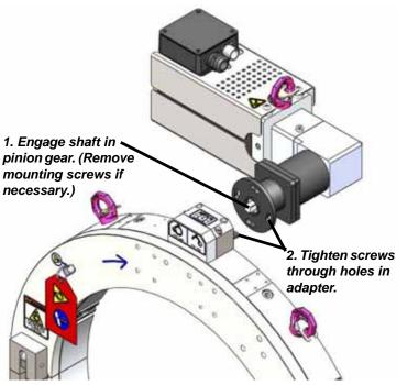
*Figure 1-6. Mount the SDE to the pinion assembly on the LCSF.*
