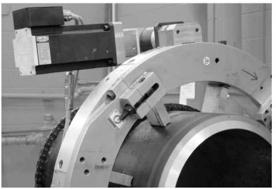
Figure 1-3. The SDE for LCSF machines is equipped with a right-angle adapter. The adapter mounts directly to the standard pinion assembly.
