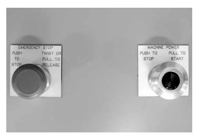
Figure 1-12. To enable the SDE, make sure the **Emer**gency Stop button is pulled out, then pull the Machine Power button. The light in the center of the button will come on to indicate power is enabled.
